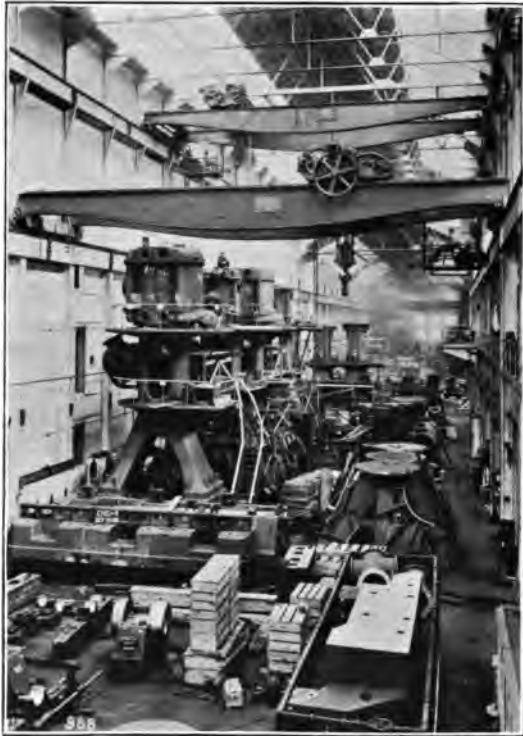
Corliss Erecting Bay
